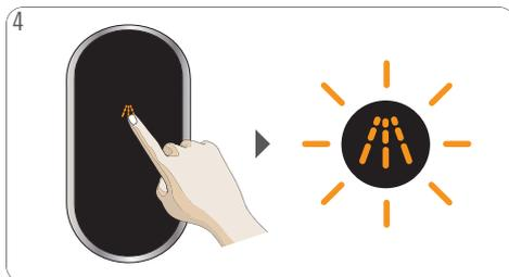
4 Touch the descaling icon for 5 seconds until the descaling LED starts blinking. The machine enters the descaling mode.
