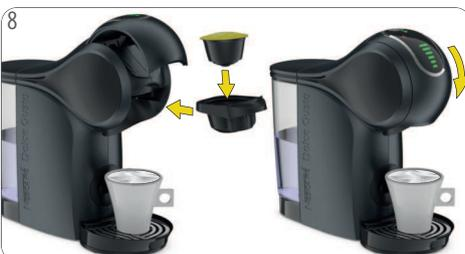
8 Insert the second capsule in the capsule holder. Insert it back into the machine. Close the locking handle.
