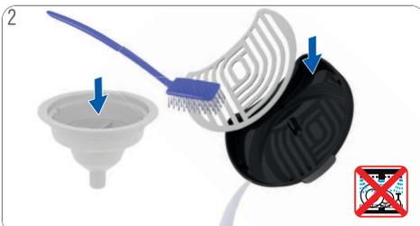
2 Rinse the drip tray and the rinsing tool with fresh drinking water. Clean the drip tray with a clean food-safe brush. The drip tray is not dishwasher safe!
