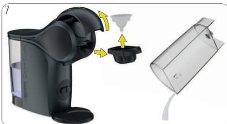
7 Open the locking handle. Pull out the capsule holder. Remove the rinsing tool. Keep it in a safe place for later cleaning or descaling. If any, remove the water from the water tank.
