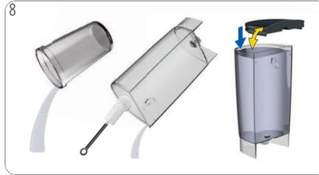
Empty and clean the container. Rinse and clean the water tank. Use a clean food-safe brush and washing-up liquid as needed. Refill the water tank with fresh drinking water and insert it into the machine. Place the container underneath the beverage outlet.
