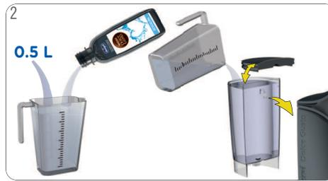
2 If any, remove the water from the water tank. Mix 0.5 liter of fresh drinking water with the descaler in a measuring cup. Pour the descaling solution into the water tank and insert the water tank into the machine.
