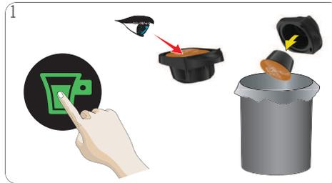
Touch the start/stop icon to stop the preparation. Pull out the capsule holder. Put the used capsule in the dustbin.
