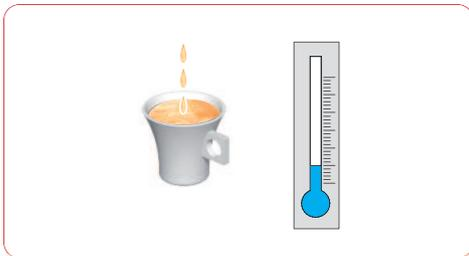
If the beverage comes out slower than usual (even in droplets), or if it is cooler than usual the machine has to be descaled.
