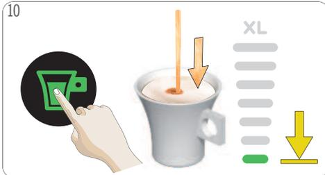
10 Touch the start/stop icon. The beverage preparation starts. **Do not open the locking handle during the extraction.** Wait until the extraction stops. The machine stops the preparation automatically. The extraction can be stopped at any time manually by pressing the start/stop icon.
