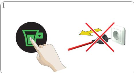
1 Always keep the machine upright! To stop the preparation, touch the start/stop icon again. Do not unplug the machine!
