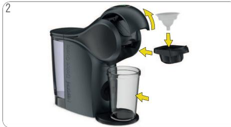
2 Open the locking handle. Put the rinsing tool into the capsule holder. Insert the capsule holder into the machine. Place a large empty container underneath the coffee outlet.
