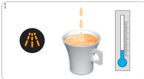
1 If the orange descaling indicator light turns on, or the beverage comes out slower than usual (even in droplets), or if it is cooler than usual, the machine has to be descaled.
