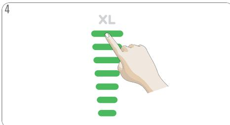
4 Set the bar display to the maximum level with the touch volume selector.
