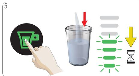
5 Touch the start/stop icon. The machine starts descaling. The bar display moves from the top down to the 4th level. The machine descales with hot water in start-stop operation. The machine stops descaling once the water tank is empty.
