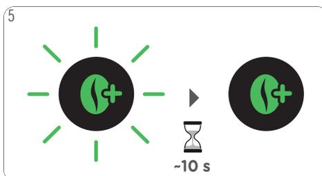
5 Pre-wetting: The preparation pauses and the ESPRESSO BOOST icon starts blinking. After approx. 10 seconds the preparation continues and the ESPRESSO BOOST icon is steady green. Wait until the machine stops automatically. The extraction can be stopped at any time manually by pressing the start/stop icon.
