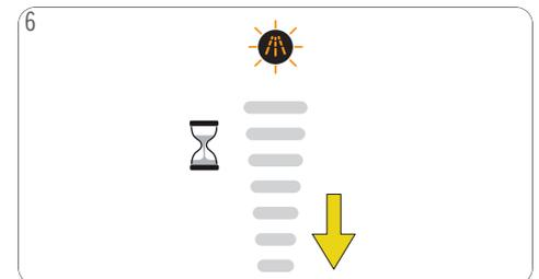
6 To allow a better descaling efficiency, the machine is on hold approximately 2 minutes. The bar display lights vanish progressively.
