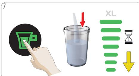
7 Touch the start/stop icon. Machine starts rinsing. Wait until the machine stops automatically. The temperature selection button and the volume display light blink for up to 8 seconds.
