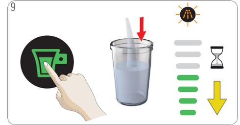
Touch the start/stop icon. The machine rinses continuously with hot water. The bar display lights vanish progressively. The machine stops rinsing once the water tank is empty.
