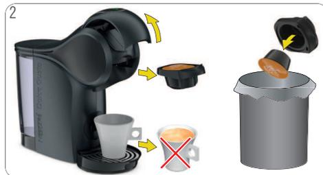
2 Do not drink the coffee! Open the locking handle. The machine releases pressure. Remove the capsule holder. Put the used capsule in the dustbin.
