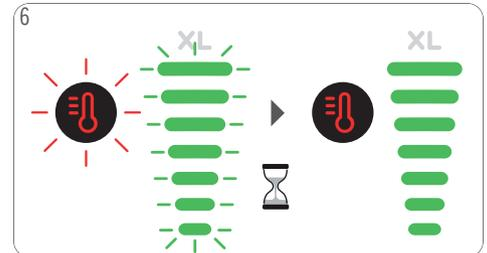
6 The temperature selection button and the volume display light blink for up to 8 seconds.
