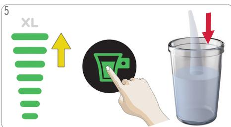
5 Set the bar display to the maximum level with the touch volume selector. Touch the start/stop icon. Machine starts rinsing.
