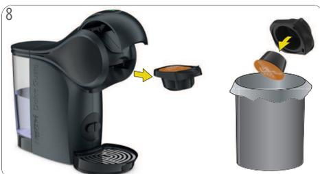
8 Pull out the capsule holder. Remove the used capsule. Put the used capsule in the dustbin.
