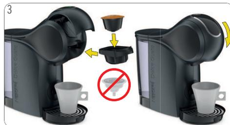
3 Make sure the rinsing tool is not inside. Insert the capsule in the capsule holder. Insert it back into the machine. Close the locking handle.
