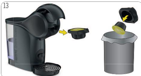
13 Pull out the capsule holder. Remove the used capsule. Put the used capsule in the dustbin.
