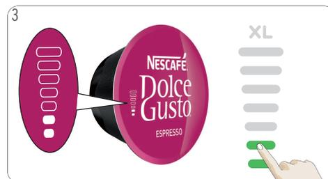
3 Use the touch volume selector to illuminate the amount of bars in accordance with the number of bars shown on the capsule, or select the amount of bars to your own taste (max level 3).
