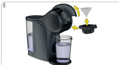
8 Open the locking handle. Pull out the rinsing tool. Reinsert the capsule holder.
