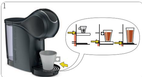
1 Adjust the drip tray position. Place the cup with the correct cup size on the drip tray. See "BEVERAGE EXAMPLES" or package. Check if the water tank contains enough fresh drinking water.
