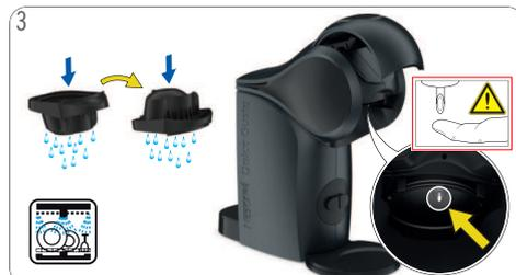
3 Clean both sides of the capsule holder with washing-up liquid and fresh drinking water. Alternatively wash in the dishwasher. Dry it afterwards. Clean the head of the machine around the injector with a clean soft damp cloth.
