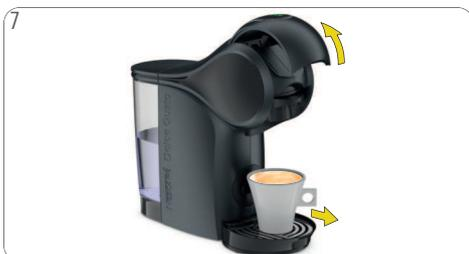
7 After the extraction is finished open the locking handle. Remove the cup from the drip tray.
