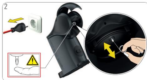
2 Remove the capsule holder. Open the locking handle. Clean the injector with the cleaning needle. Follow instructions in 9. "DESCALING AT LEAST EVERY 3–4 MONTHS" on page 18.
