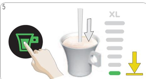
5 Touch the start/stop icon. The beverage preparation starts. **Do not open the locking handle during the extraction.** Wait until the extraction stops. The machine stops the preparation automatically. The extraction can be stopped at any time manually by pressing the start/stop icon.
