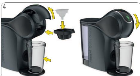
4 Open the locking handle. Put the rinsing tool into the capsule holder. Insert the capsule holder into the machine. Close the locking handle. Remove the drip tray. Place a large empty container underneath the coffee outlet.
