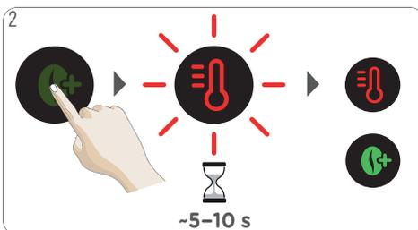
2 Touch the ESPRESSO BOOST icon to switch to ESPRESSO BOOST. The temperature selection icon blinks while the machine is heating up for approximately 5–10 seconds. Afterwards, the temperature selection icon lights steady red. The machine is ready to be used.
