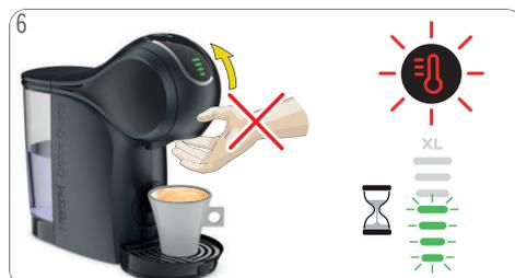
6 After finishing the preparation, the temperature selection icon and the bar display light blink for up to 8 seconds. **During that time do not open the locking handle!**
