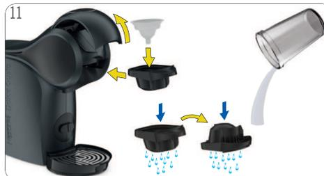
Remove the container. Empty and clean the container. Pull out the capsule holder. Remove the rinsing tool. Keep it in a safe place for later cleaning or descaling. Rinse both sides of the capsule holder with fresh drinking water. Reinsert the capsule holder.
