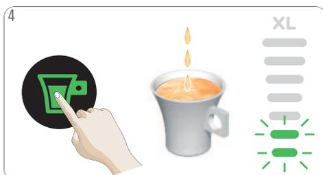
4 Touch the start/stop icon. The beverage preparation starts. **Do not open the locking handle during the extraction.**
